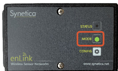
Blinking Green LED - Device Successfully Joined
