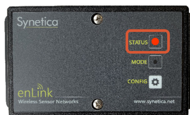
Blinking Red LED - Attempting to Join
