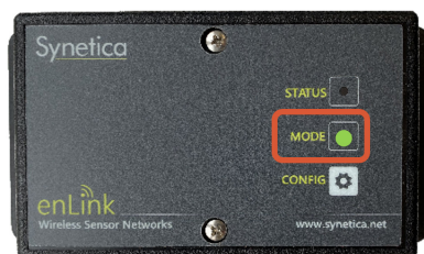
Blinking Green LED - Device Successfully Joined
