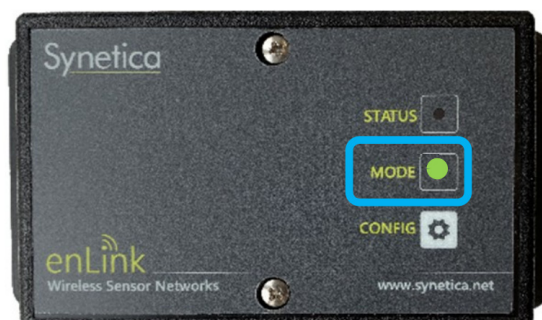
Blinking Green LED - Device Successfully Joined
