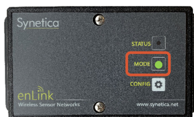
Blinking Green LED - Device Successfully Joined
